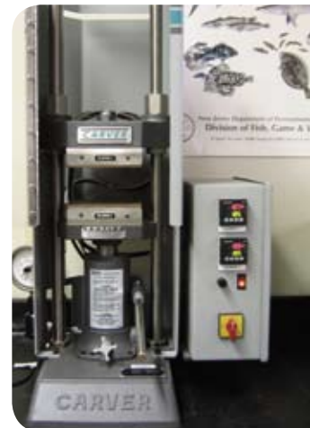
Fish scales are heated in this press to burn an impression onto an acetate slide.
